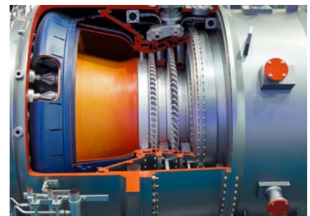
Example: power supply Non-contact displacement sensors monitor the blade gap, enabling low-wear and long-term operation in gas turbines.
