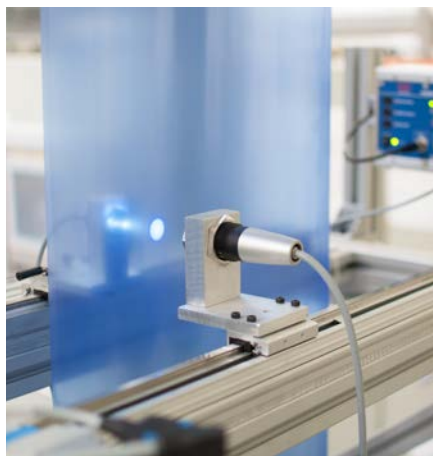
Inline color gradient measurement of transparent film and acrylic glasses.
