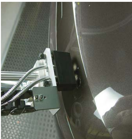
Detection of the color identity of attachments in automotive manufacturing.
