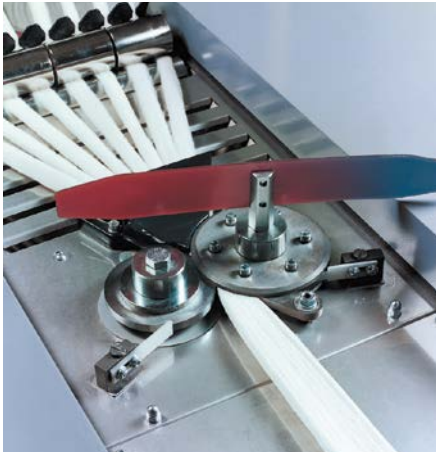
Inline yarn thickness measurement
