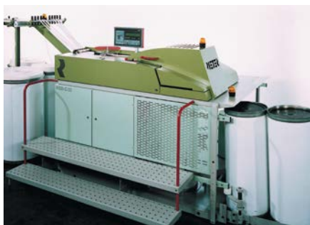
Example: machine monitoring Eddy current sensors monitor the fluctuating thickness of yarns in textile machines.
