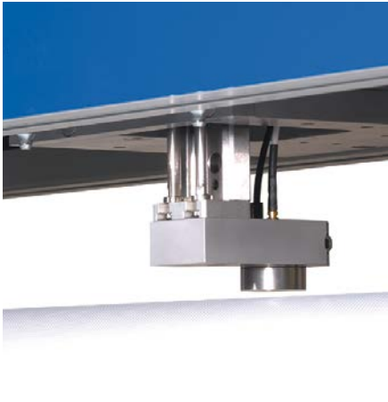
Non-contact, inline thickness measurement of plastic films
