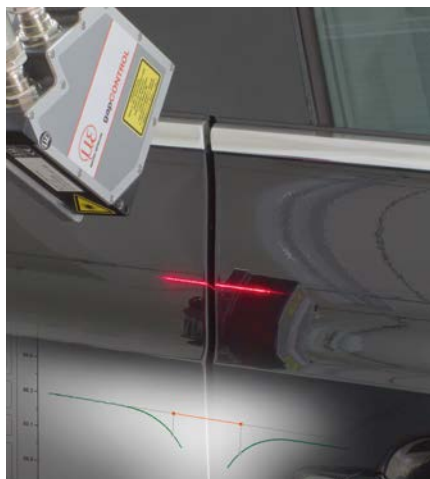
Gap and flushness measurement on bodywork parts
