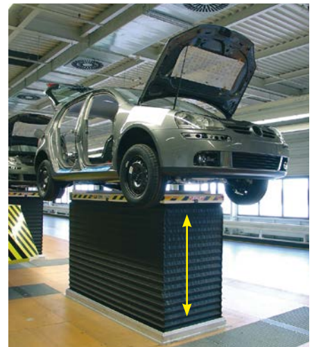
Customer-specific draw-wire sensors as important OEM component: Draw-wire sensors monitor the height of lifting platforms on automobile production lines.
