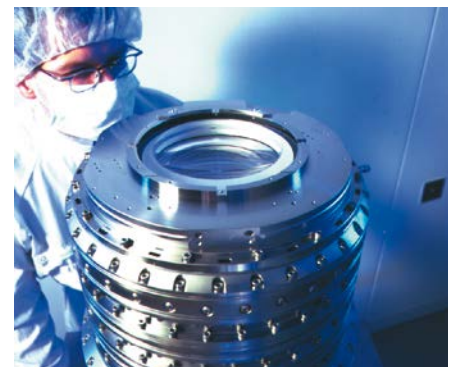
Non-contact, capacitive displacement sensors are used for nanometer adjustments of lenses in objectives for wafer exposures.
