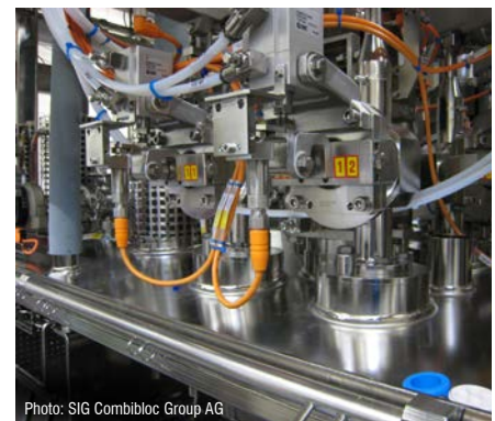
Valve lift measurement in the food industry The sealed stainless steel housings of the MDS-45-Mxx series are ideal for the food industry.
